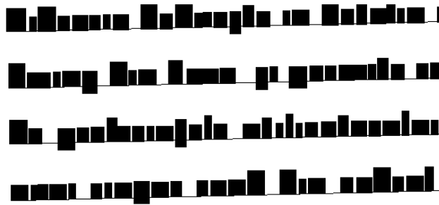
Fig. 7. Characters represented by their bounding boxes, clustered together. The line at the bottom is the identified skew line
