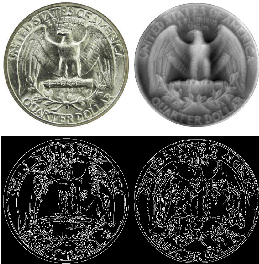
Fig. 14. Diffuse image (left) vs Depth map (right - taken from [29]) - the edge detection is more uniform for the depth map
