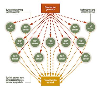
As we can understand from the picture above, DRDoS is the worst type DoS Attack, because it uses valid TCP connections from valid hosts.
