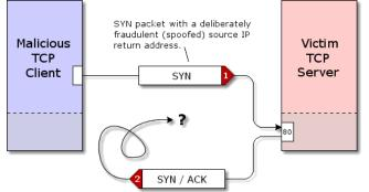
The packet's "return address" (source IP) can be overridden and falsified. When a SYN packet with a spoofed source IP arrives at the server, it appears as any other valid connection request. The server will
