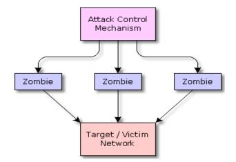
The diagram above shows the architecture commonly used in distributed denial of service attacks. The operation of a network of compromised machines, containing remotely controlled "Zombie" attack programs, is directed and coordinated by a "Zombie Master" central control agency. When the network of Zombies receives instructions from its Master, each individual Zombie begins generating a flood of malicious traffic aimed at a single target/victim machine or network.
