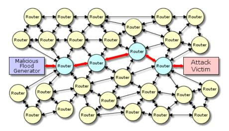
The Internet is essentially a large network of individual, interconnected, packet routers. The specific path taken by individual packets moving between any two Internet endpoints may change as a result of local network outages, congested routers, and other factors. However, over a short period of time, most packets will travel along the "best path" — which rarely changes from one packet to the next.
