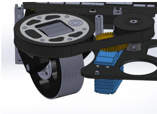
Figure 7. Servomotor connected to the module through two transmissions.
