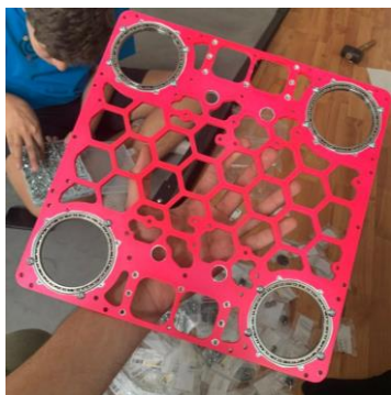
Figure 23. X-contact Bearings are mounted to the main plate.
