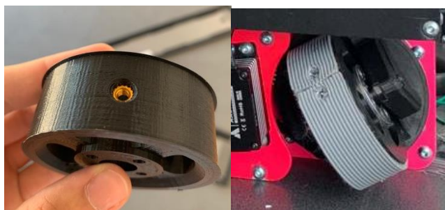
Figure 20. Threaded heat inserts mounted in the 3D printed wheel rim.
