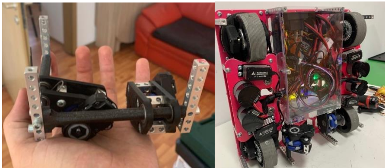
Figure 27. The odometry subassembly
