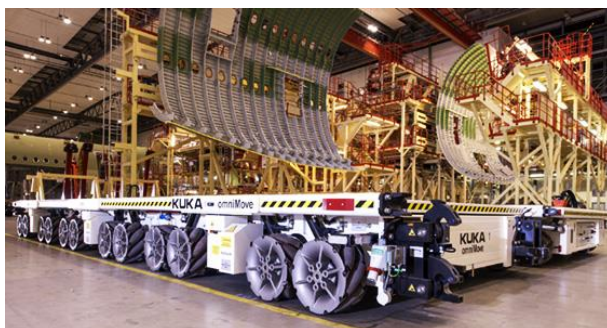
Figure 1. Mecanum transporter for Airbus components 3 .
