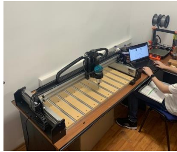
Figure 19. The CNC machine and one 3D printer used in the manufacturing process.
