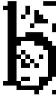
Figure 2. An encompassing rectangle around a binarized letter b
