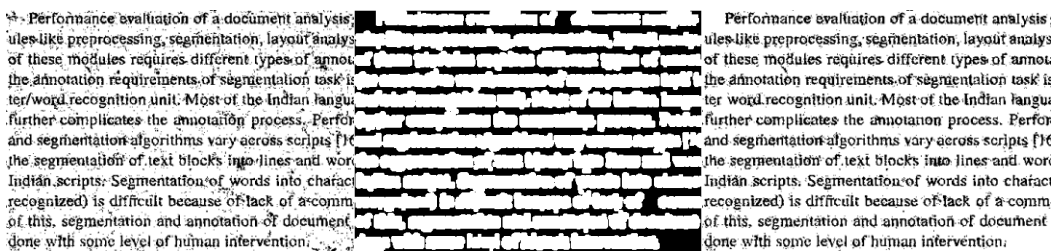
Figure 10. The final result (right) obtained after combining the binary image (left) with the dilated gradient map (center).
