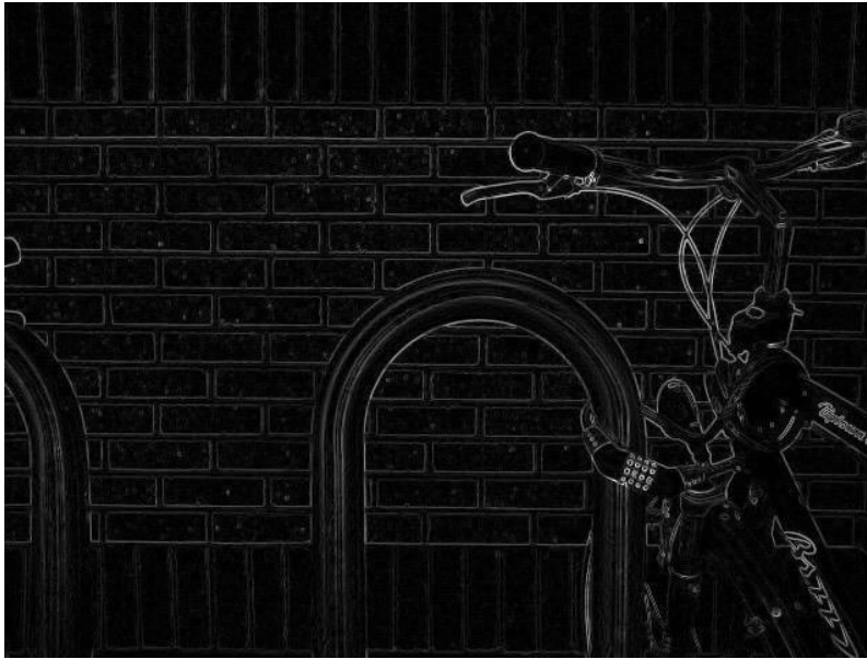
Figure 2. Gradient magnitude from Robert cross operator [13]
