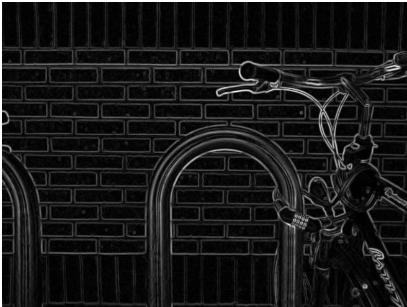
Figure 4. Gradient magnitude from Sobel operator [15]
